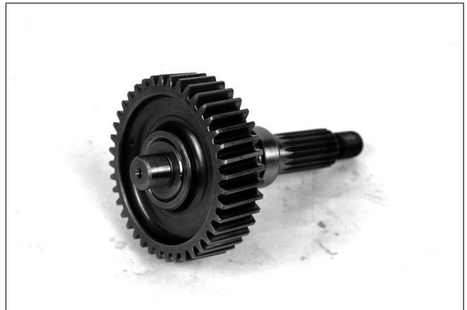
Check the countershaft for wear or damage.
