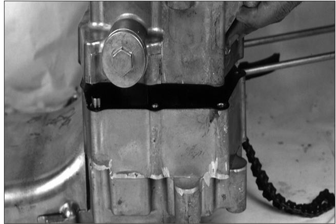
Tighten the crank case bolts.
