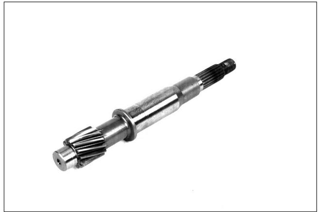
Check the final shaft for wear or damage.
